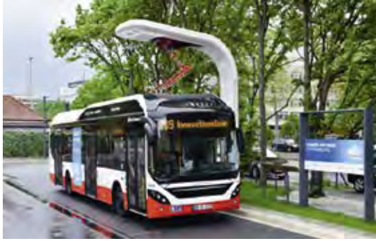
Plug-in bus at the electric bus terminal on Adenauerallee
